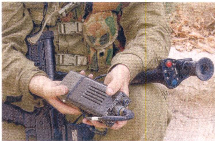
■ Cornerstone of ITL's AISS soldier ensemble is the micro tactical computer (centre), which is operated via the associated handheld display (right).
